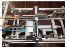
Important - Always place each actuator in the right socket of the controller. After each replacement of a new Actuator, or if a plug of any actuator was taken out - a RESET must be preformed.
