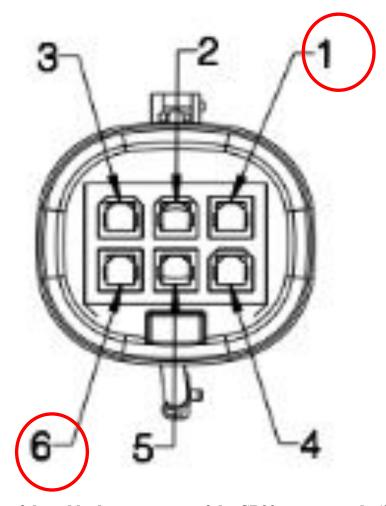
This is the front view of the cable that comes out of the CB20 power supply (first socket in the CB20).
